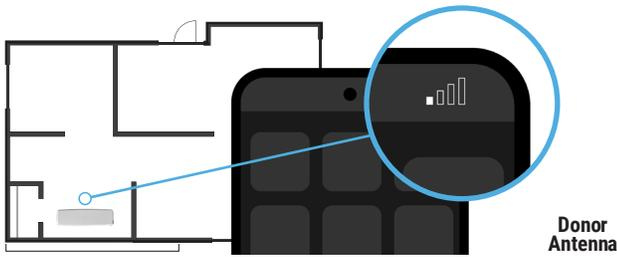
Use your phone to find where coverage is needed. This is where the **Server Antenna** should be installed on a wall.
