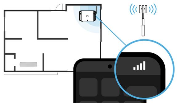
Place the **Main Unit** near a window where there is a strong signal. Ideally, the **Main Unit** should be placed with at least one wall from the **Server Antenna** and as far as the cable will allow. If the **Server Antenna** cable is too short, it can be extended with a separate coaxial cable having SMA(m) & SMA(f) connectors.
